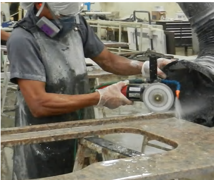
Wet methods and dust-capture systems are safer for workers.
